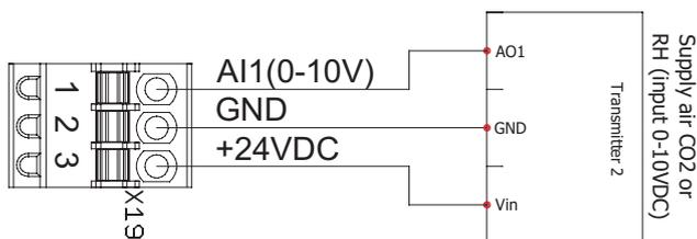
**21.5. EXTRACT AIR CO<sub>2</sub> OR RH (INPUT 0-10VDC)**
