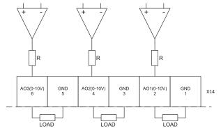
MCB V2.0 PWM 0-10V, 1kHz; MCB V2.0 Analog voltage 0-10V;  $R{=}510~\Omega$
