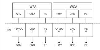
WPA - Water preheater actuator WCA - Water heater actuator
