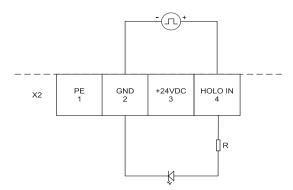
$R = 1 \text{ k}\Omega$ ;  $U_f = 1.5 \text{ V}$ ;  $I_f min. = 1 \text{ mA}$ ;  $I_f max. = 50 \text{ mA}$
