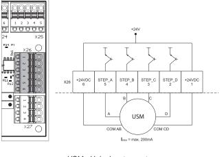
USM - Unipolar step motor
