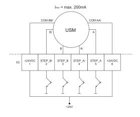
USM - unipolar step motor
